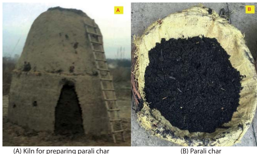
Figure 1: Indigenous technique of preparing parali char
